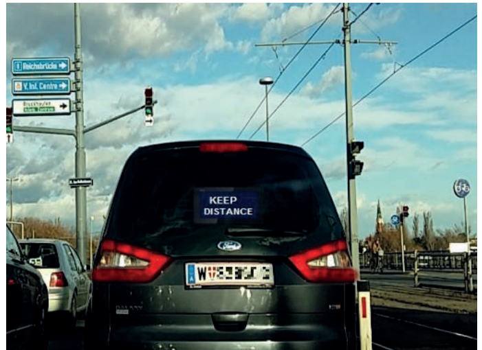
Figure 2. Message displayed to the tailgating vehicle
