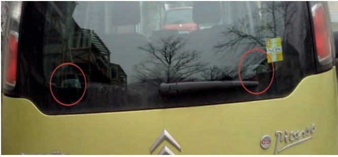
Figure 3. Location of the cameras in the rear part of the vehicle.
