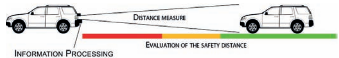
Figure 1. Cooperative driving in which visual data related to the safety distance is provided to the vehicle behind in real-time
