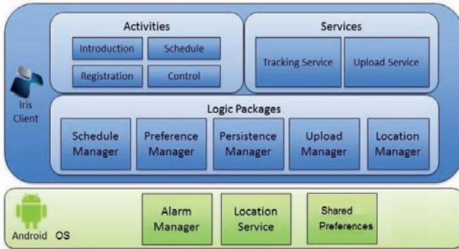
Fig. 5. Client side of the Iris system architecture.
