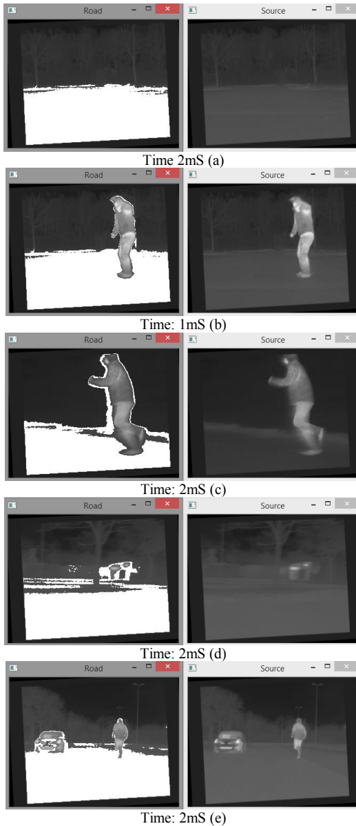
Figure 1(a) to (e): Execution time and results of the chromatic algorithm. The images on the left image show the results in white. The images on the right are the source images that have not yet been processed.
