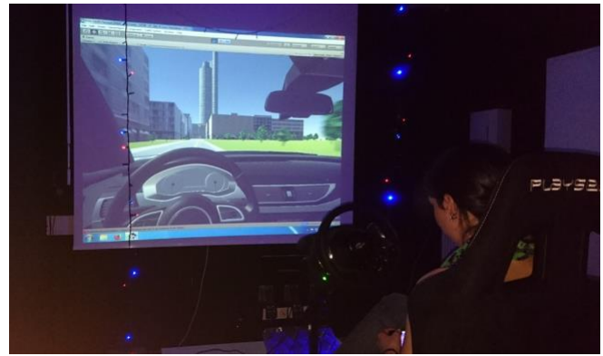
Figure 4. Simulation set up showing the luminescence as visual stimulus.
