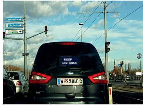
Fig. 5. Urgency cue related to safety distance provided to the rear vehicle in real-time [50].
