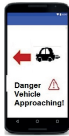
Fig. 4. Object cue in combination with direction cue that warns a VRU about a vehicle in the immediate vicinity, and states the position of the danger [51].
