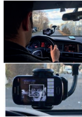
Fig. 1. In-vehicle location of the smart phone for a smooth face characteristics detection
